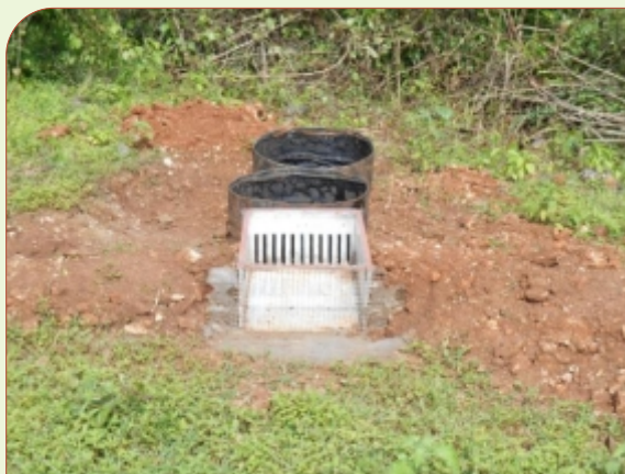
MSD fitted with drums for runoff & soil loss monitoring
